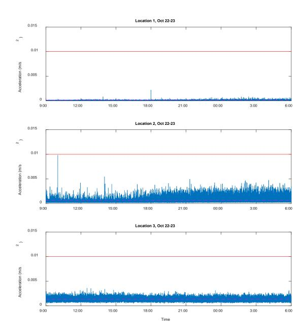
Figure 1: RMS particle accelerations at Location 1, 2 and 3 on October 22-23, 2017. The magenta dash line represents the mean baseline rms particle acceleration calculated from October 5 to 16 at each location. The red line shows the  $0.01 \, \text{m/s}^2$  threshold of the RMS particle acceleration.
